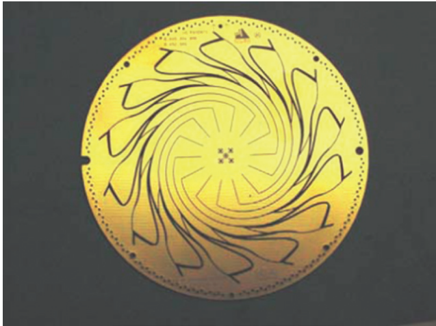
Fig. 5.14 Enhanced pinwheel GNSS antenna (radome removed) plane [35] (courtesy of NovAtel).
